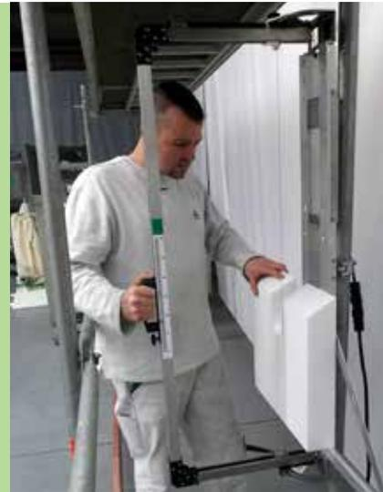
The **inoCUT ic2** revolutionises the thermal cutting of ETICS rigid foam panels on the construction site. The space-saving cutting bracket guarantees maximum freedom of movement and a sufficient route of approx. 20 cm on the scaffold (for a scaffold width of W06). Unlike conventional devices, the cutting bracket does not have to be pulled out to double the width for cutting operations. The cutting wire moves within the compact bracket thanks to its unique mechanism.
