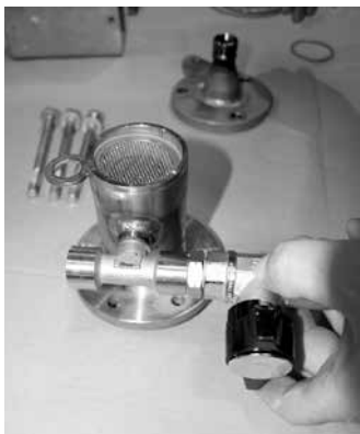
1. Insert the paint strainer in the centre piece. Then place the centre piece on the pressure flange with the check valve.
