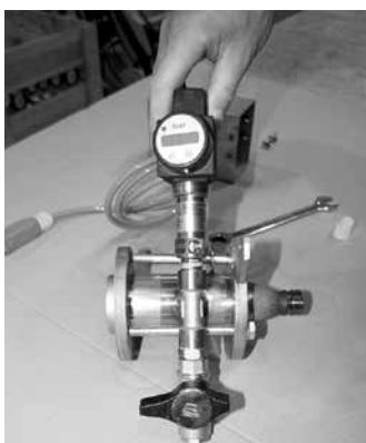
4. Screw the pressure sensor onto the pressure gauge receptacle.
