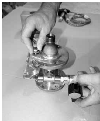
3. Insert the three screws (M10 x 120)...
