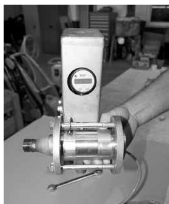
... and connect it to the housing bracket on the outlet flange with two screws (M6 x 20)
