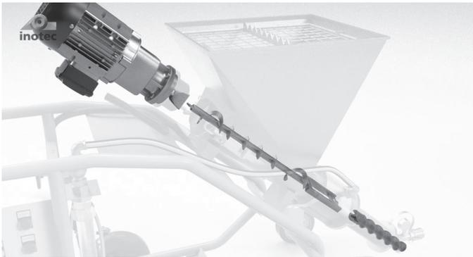
This sectional image illustrates the connection from the motor to the mixing coil, and from the mixing coil to the pump unit (rotor/stator).
