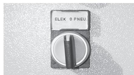
Switch for electrical or pneumatic control of the machine.
