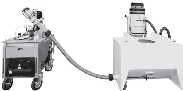
Material loading of a mixing pump from a Big-Bag-Box Mono with the inoFLEX Mono dry conveying unit.
