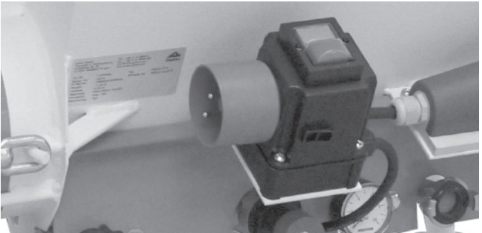
Connector plug on the On/Off switch
